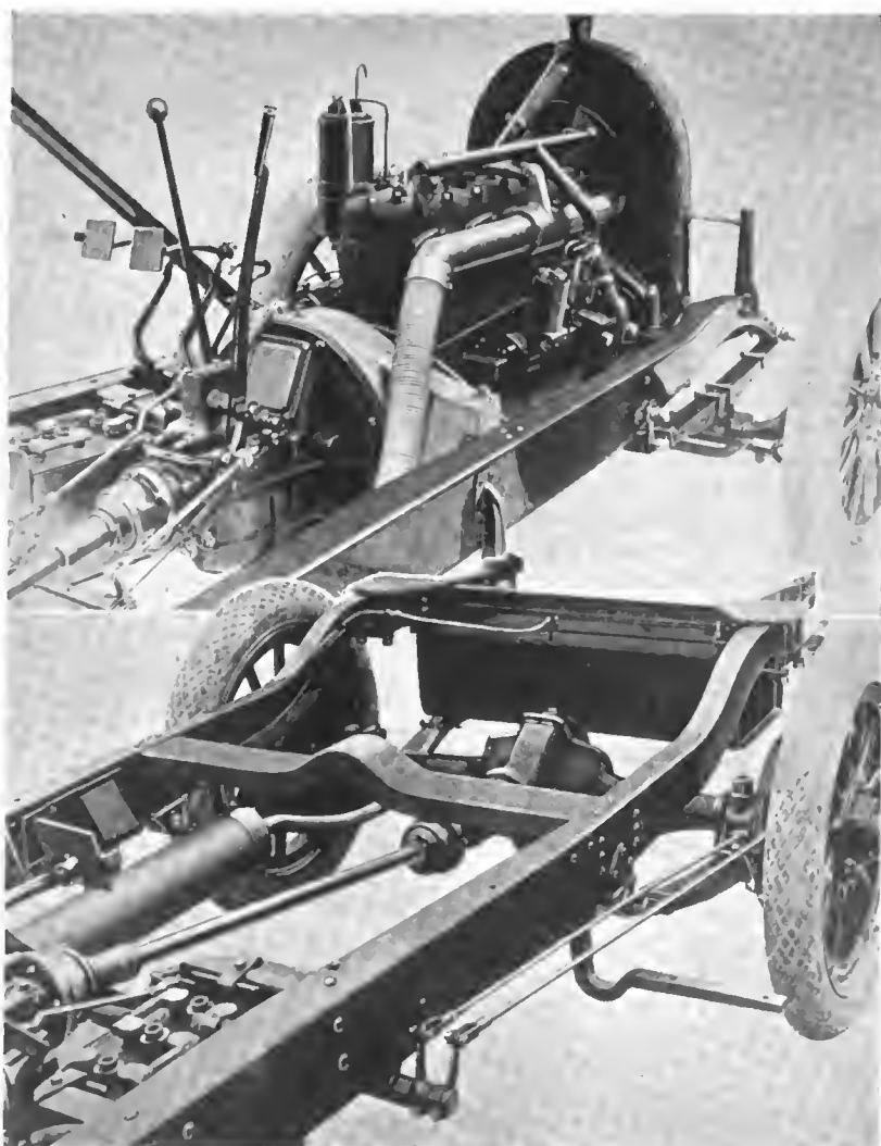
Two chassis views. Note the mounting of the Stewart vacuum fuel feed system, the flexible exhaust line and the deep section frame. Also the battery mounting and the speedometer drive off the rear of the gearbox
